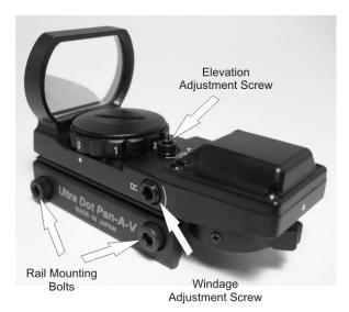
Make certain that you loosen your wind/elev locking screw before making adjustments to your sight. After sighting in has been completed, retighten the locking screw to prevent your sight from moving. Be careful not to over-tighten the locking screw.
